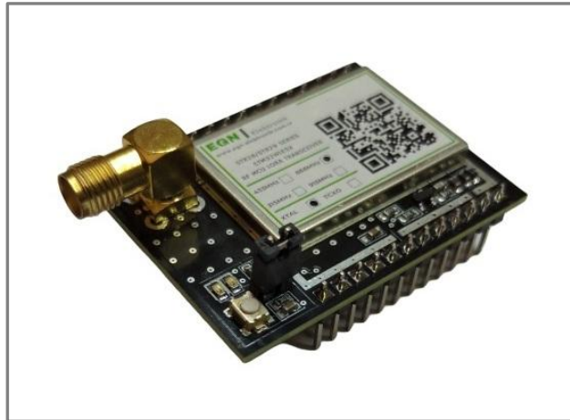
Fig.2 STR29RSH3 315MHz/+20dBm RF LoRa Transceiver Module
